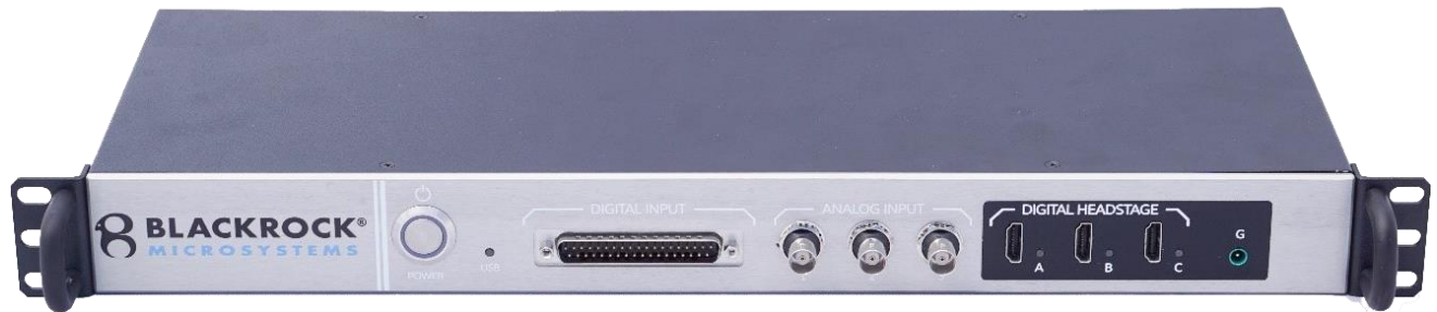
CerePlex Direct front panel. From left to right: Power switch, USB LED, 16-bit digital input, analog input BNC connectors, digital headstage HDMI inputs (with LEDs), touchproof patient ground connector
