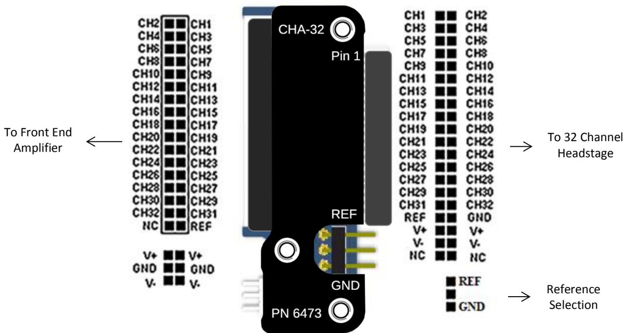
**Figure 1: CHA-32 Board Pin-Out**
