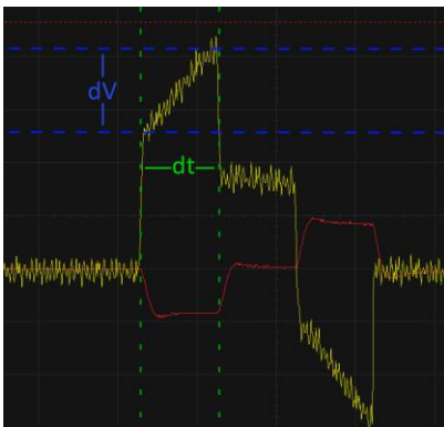
Figure 1-Oscilloscope trace of the monitor port. Stimulation current shown in red, stimulation voltage shown in yellow
