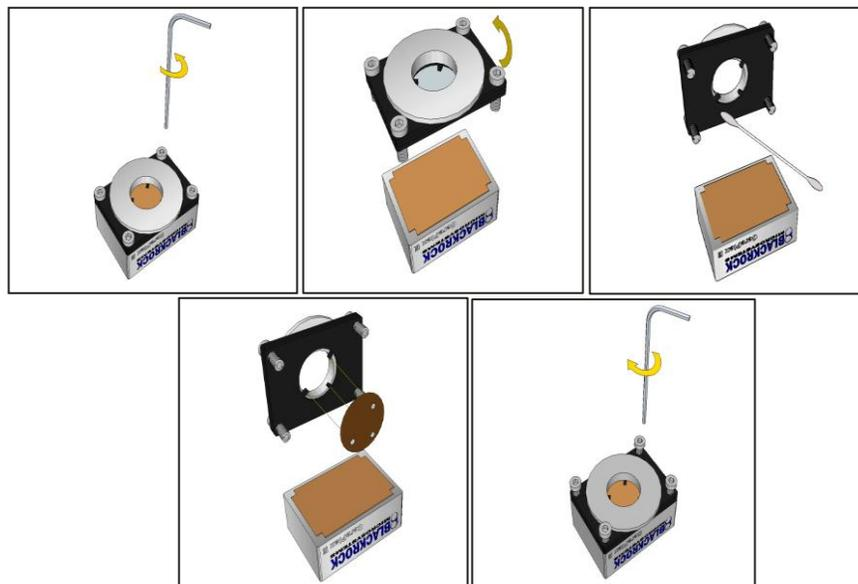
Figure 6- Replacing the Filament Film
