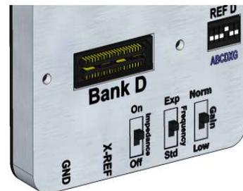
Figure 5–CerePlex A Impedance DIP Switch
