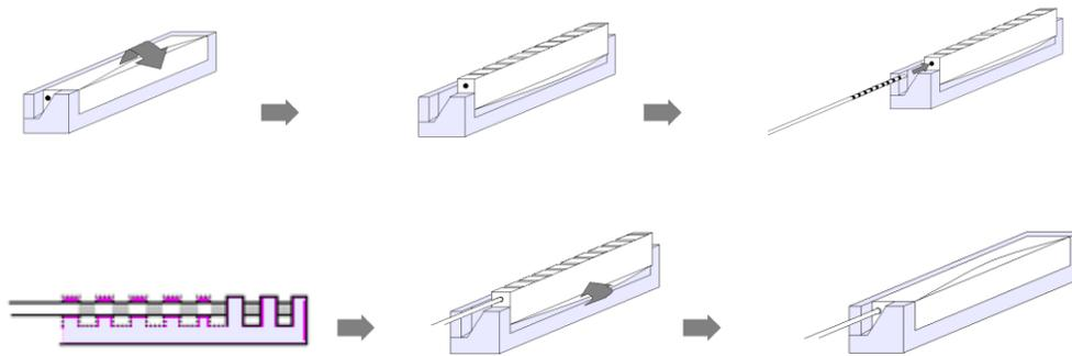
**Figure 3—Connecting the pigtail to the Cabrio Connector. After the pigtail is inserted, make sure the contacts on the pigtail are correctly placed in-between the intervals on the connector.**
