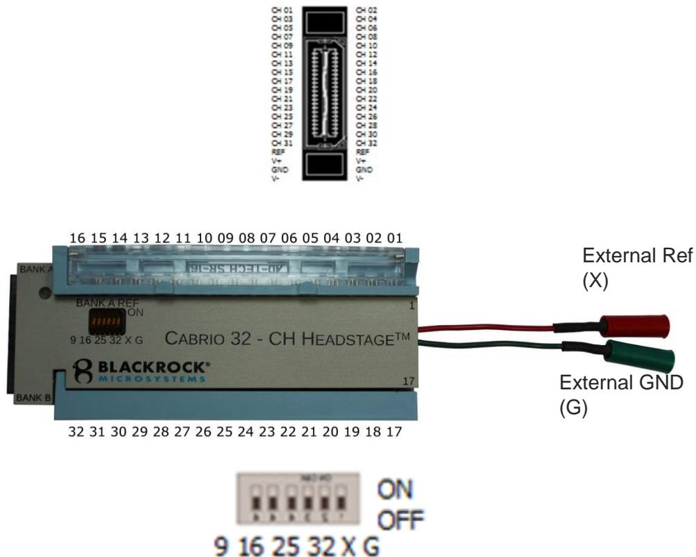
Figure 2—Blackrock 32-Channel Cabrio Butterfly Ref Adapter Pin-Out
