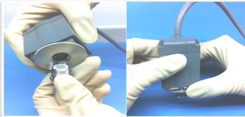
Figure 5 - Attaching the Patient Cable
